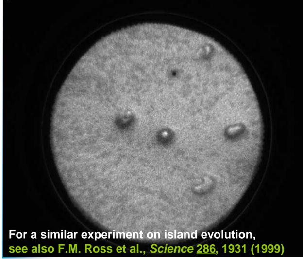
8 ML Ge on Si(111) **LEEM Movie:** post-deposition annealing to 550° C **Bottom right:** an unstable island "melts" **Upper left:** an island nucleates, then is divided in 2 **FoV:** ~5 μm
