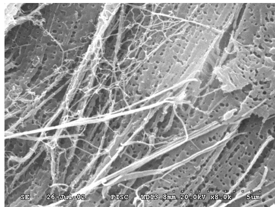
Figure 4 SEM photograph of fibrils on the surface of the hybrid board, magnification × 8000.
