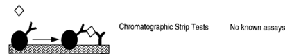
Fig. 4 "One Step" strip or chromatographic tests and assays. First antibody-coated, dyed microspheres migrate along strip to immobilized second antibody; antigen sandwich forms colored line.
