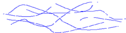
This is what polymer chains look like in a piece of stretched rubber. Entropy does not like this.
