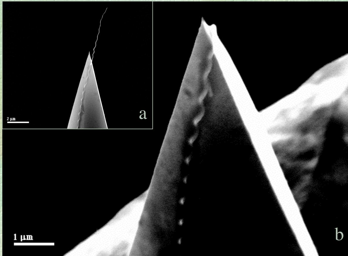
a) MWNT probe. b) MWNT probe after immersion in H<sub>2</sub>O. MWNT is folded back against the underlying Si probe where it is pinned against this surface by Van der Waals forces.
