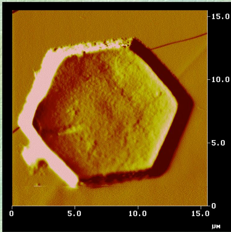
HSP 60 protein crystal imaged using MWCNT probe in air.
