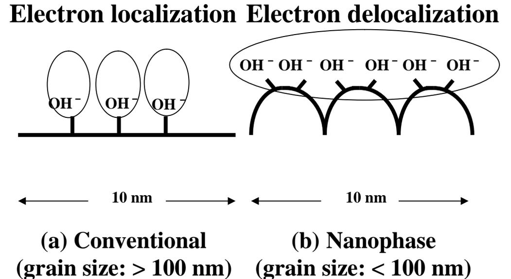
Nanophase materials have higher surface areas, possess greater numbers of atoms at the surface, altered electron delocalization, etc\*.
