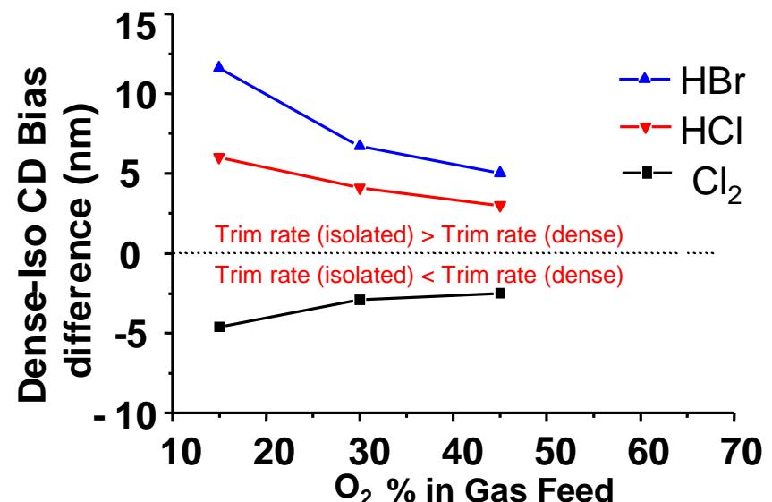
$$CD \text{ Bias} = CD_{\text{after trimming}} - CD_{\text{before trimming}}$$
