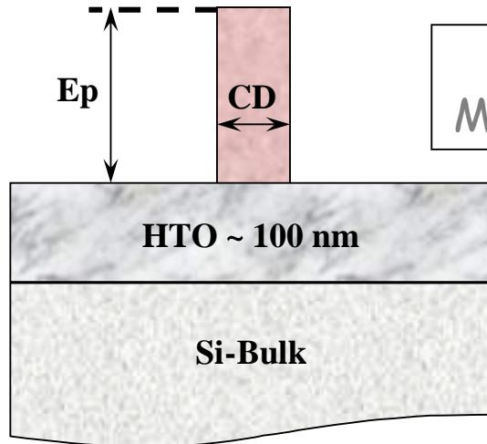
$$\text{CD Bias} = \text{CD}_{\text{before trimming}} - \text{CD}_{\text{after trimming}}$$
