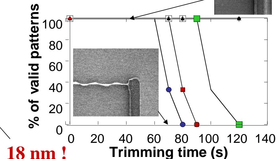
Limit width after trimming for a yield of 100% : 22-23 nm
